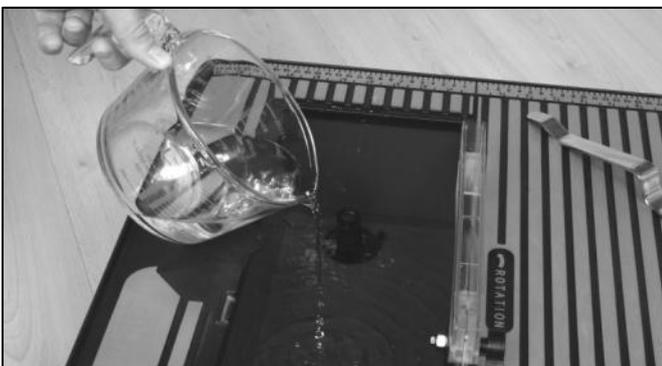
Fill the reservoir to a point just below the overflow opening at the top of the drain plug. Replace cutting table. Check frequently during use – do not allow the blade to run dry.
