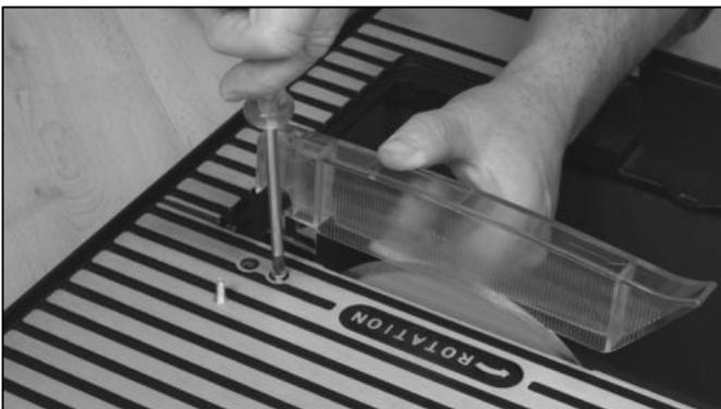
Before replacing table top, fasten guard support in the slot behind the blade opening using the screws provided. Attach the blade guard to the support using bolt and wing nut.
