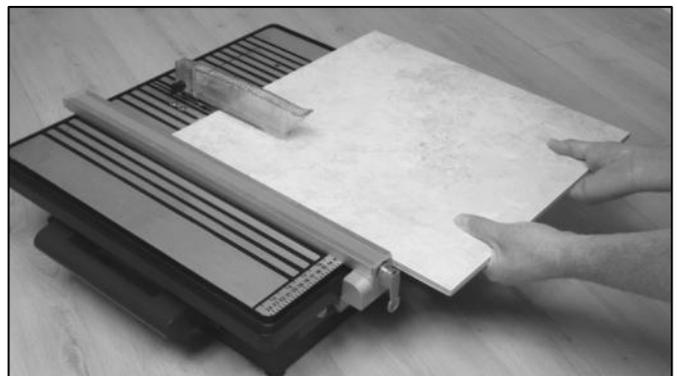
Maintain an even pressure, hold the tile against the cutting guide and push steadily through the cutting wheel. When the cut is complete, then switch off the machine.
