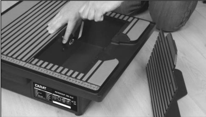
To fit or replace the cutting wheel, first take out the removable side of the cutting table. Remove nut and washer using the wrench provided.
