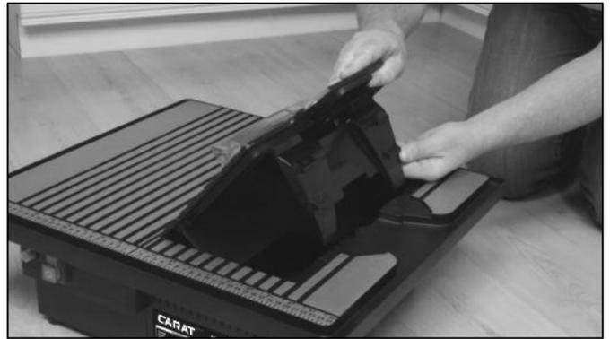
For mitre cuts, raise the cutting table to the required angle (15, 30 or 45 degrees)
