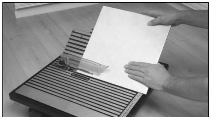
Switch on the machine and feed the tile through the cutting wheel. When the cut is complete, switch off the machine.
