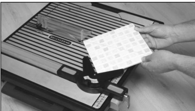
Re-tighten the knob and position the tile within the jaws of the mitre guide.
