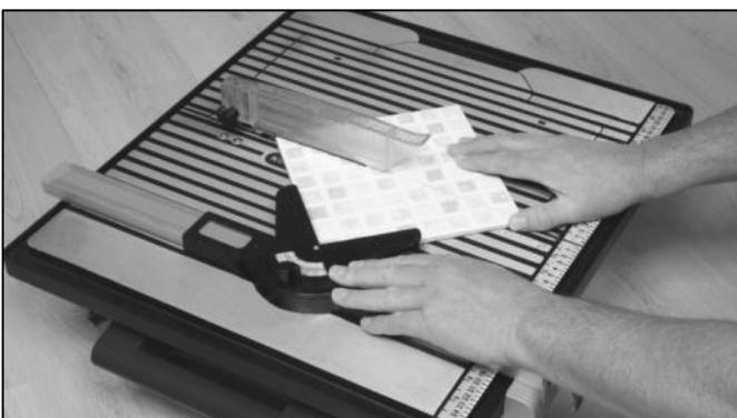
Switch on the machine and while holding the tile firmly in position, push the mitre guide steadily along the rip guide, feeding the tile through the cutting wheel. When the cut is complete, switch off the machine.
