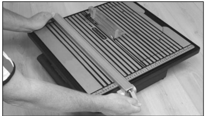
Place the Rip Guide on the preferred side of the table top and line up with the rule edge to the required measurement of the tile to be cut. When correctly aligned, lock in place by pushing the adjuster firmly downwards.
