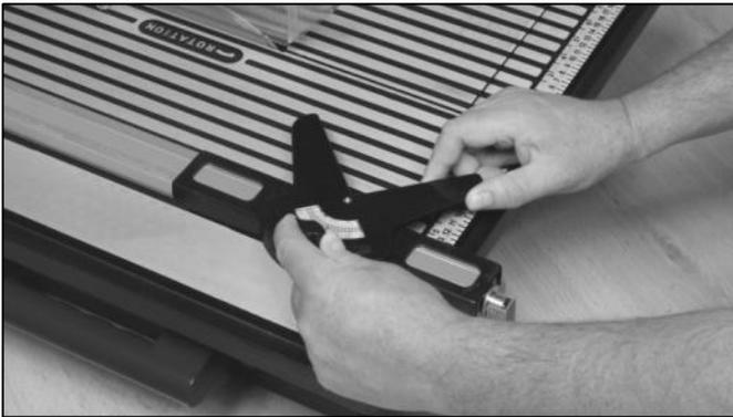
Slacken the thumb screw and set the required angle of cut.
