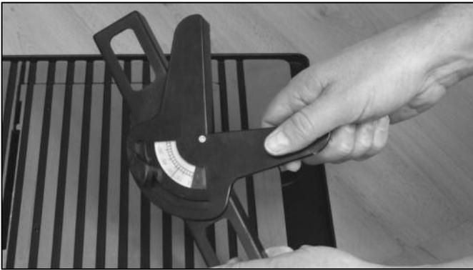
Slide the mitre guide into place on the rip guide.
